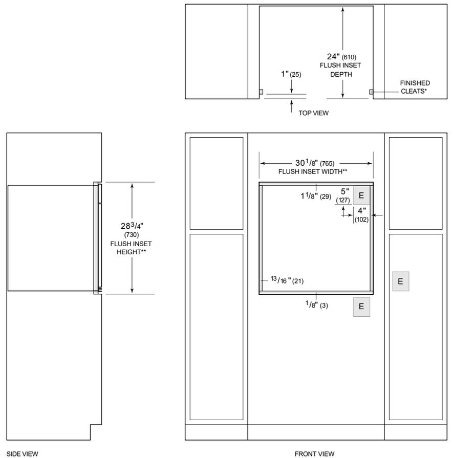
\*1" (25) minimum depth. Shaded areas will be visible and should be finished to match cabinetry.
