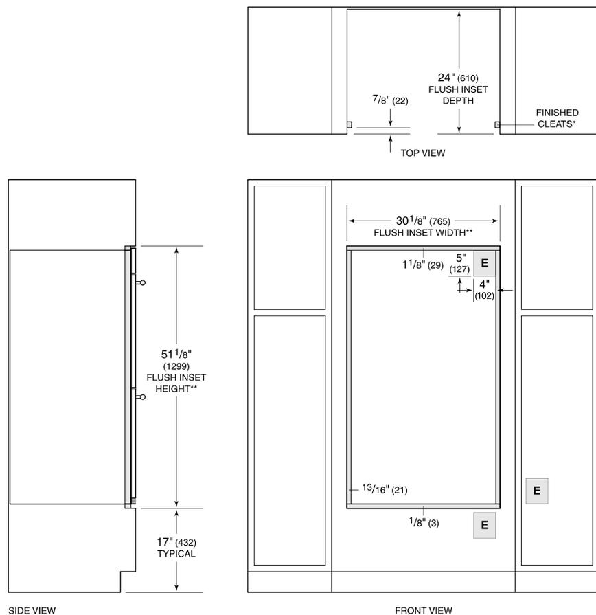
\*1" (25) minimum depth. Shaded areas will be visible and should be finished to match cabinetry.
