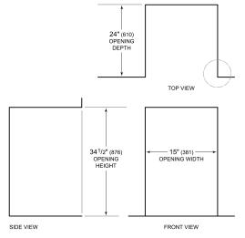
NOTE:  $3^{1}/2^{m}$  (89) finished returns will be visible and should be finished to match cabinetry.
