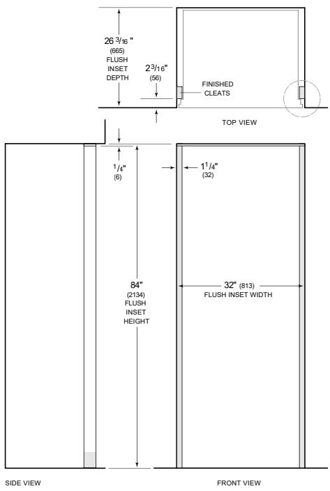
NOTE: 3 1/2" (89) finished returns and shaded areas will be visible and should be finished to match cabinetry. Shaded line represents profile of unit to 1 1/4" (32) panel.
