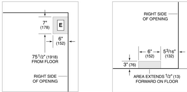
**NOTE:** Dimensions in parenthesis are in millimeters unless otherwise specified
