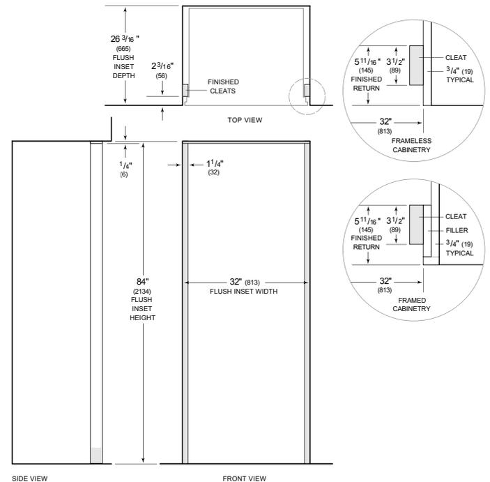
**NOTE:** 3 1/2" (89) finished returns and shaded areas will be visible and should be finished to match cabinetry. Shaded line represents profile of unit with 1/4" (19) panel.
