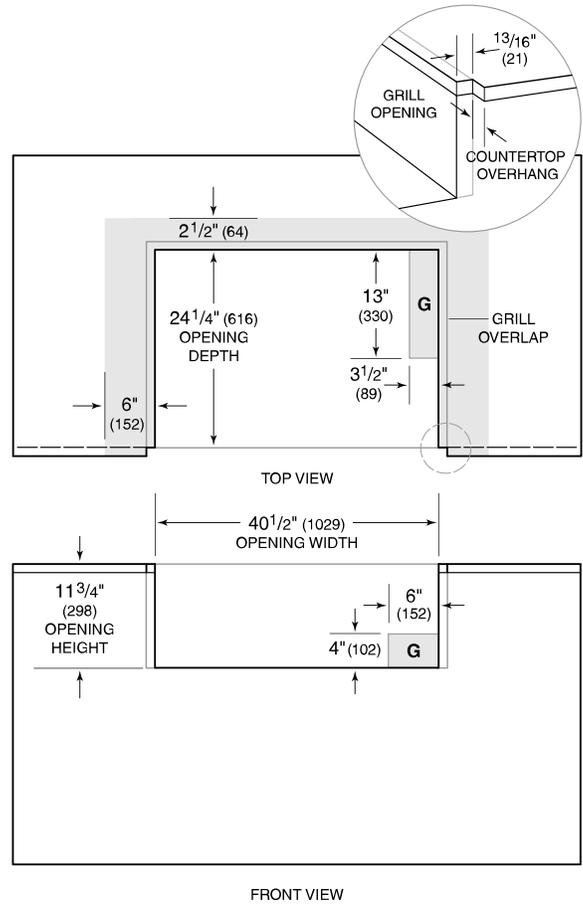
NOTE: Shaded area above countertop indicates minimum clearance to combustibles, combustibles cannot be located within this area.
