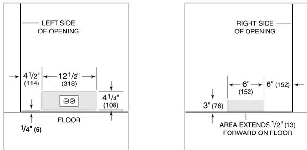
**NOTE:** The electrical outlet must be positioned with the grounding prong to the right of the thinner blades.
