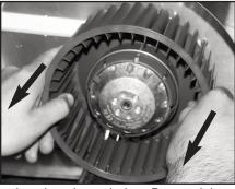
Install 4 screws into the location shown below. Do not tighten screws down fully, leave a 1/8" gap. Hang blower unit onto blower plate (screws through the large part of the keyholes. Slide the blower to its position (screws in the small part of the keyhole). Tighten the screws.
